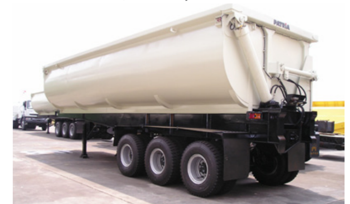
SDT 85T mining trailer with York 17.5T and YTE 90 suspension.
