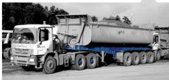
These side tippers have a capacity in excess of 100 tonnes.
