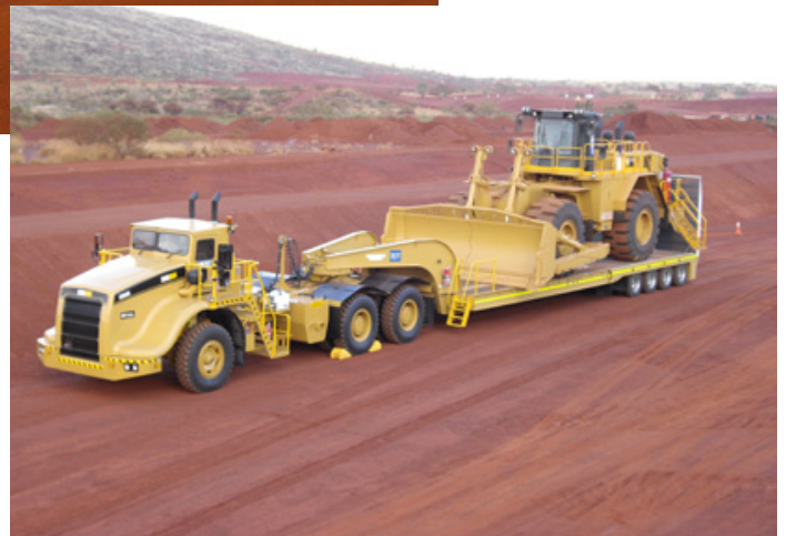
Below: Drake has added a new mine site trailer to its range of specialised transport equipment. These smaller capacity trailers are designed to carry machines and equipment between the 100 to 200 tonne range.
