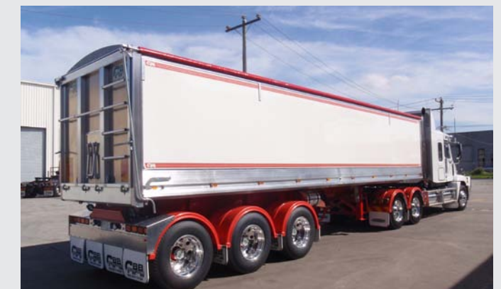
Loyal supplier: A Chris's Body Builders B-Trailer with tri-axle York Duratec air ride suspension and premium Baron axles.
