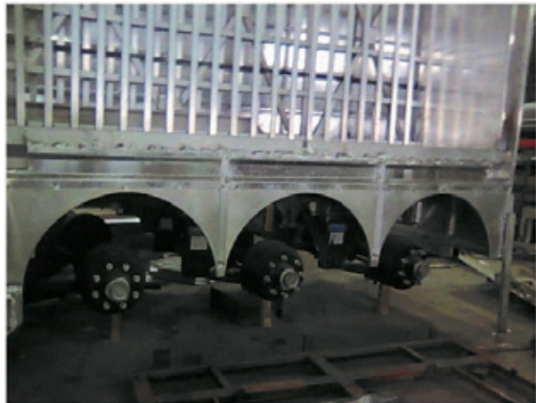
3 x Tec Air 1 - 12 ton Capacity suspensions
