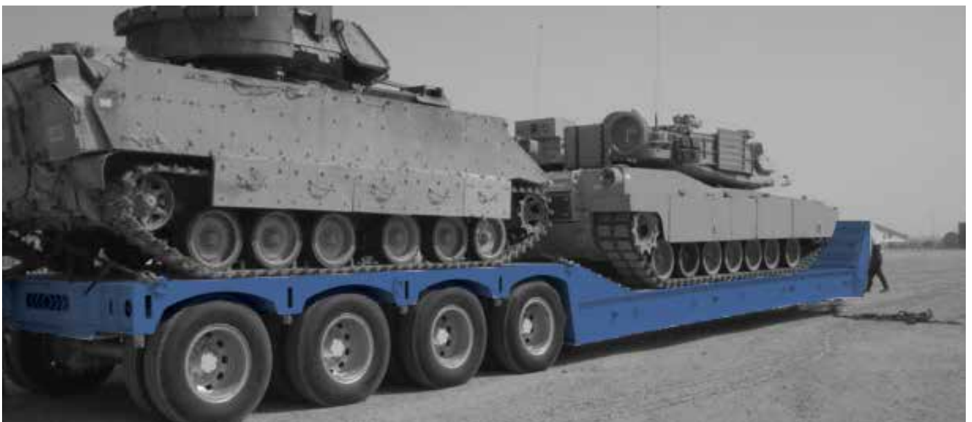
Army tank being carried on vehicles fitted with York axle & suspension.
